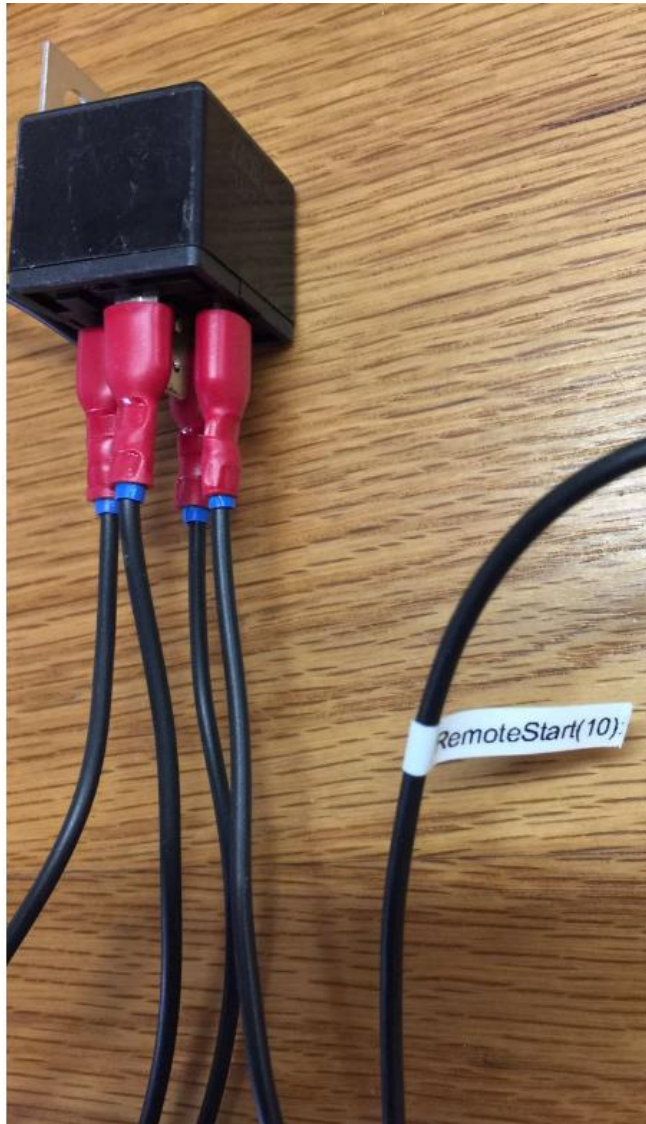
Figure 3 - Output1 Relay for remote start
